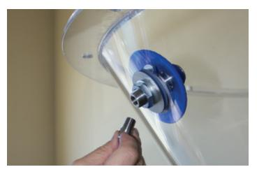
**7.** Tighten to the specified fluidizer torque of 25 ft. lbs (35 Nm) and remove the retaining cable.
