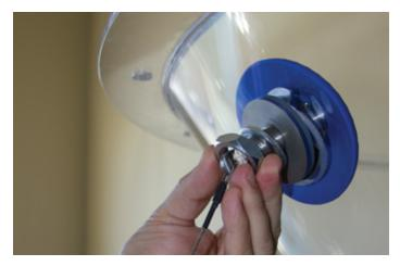
**6.** While continuing to hold retaining cable, slide the Fast-Fit<sup>™</sup> sealing washer and the Fluidizer washer over the retaining cable and onto the stem. Next slide the nut over the retaining cable and thread it onto the stem.
