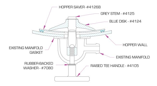
\*\*\*The replacement parts above incorporate the existing manifold and manifold gasket. In order to receive the maximum benefit of the Solimar Trailer Fluidizer system, we recommend using the Solimar manifold, which is ported for  $1-\frac{1}{2}$ " and 2" air lines.
