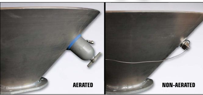
Converting an aerated hopper to non-aerated discharge is now easy with the new Hopper Plug from Solimar. This high quality solution replaces aerators for sugar hauling, pneumatic trailers and vacuum, plastic pellet tanks. The aluminum plug comes with a threaded end to slide through the hole left by an aerator in the hopper bottom. A stainless steel lock washer and nut are included to
