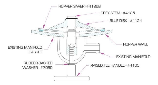
\* \* \*The replacement parts above incorporate the existing manifold and manifold gasket. In order to receive the maximum benefit of the Solimar Trailer Fluidizer system, we recommend using the Solimar manifold, which is ported for 1-1/2" and 2" air lines.
