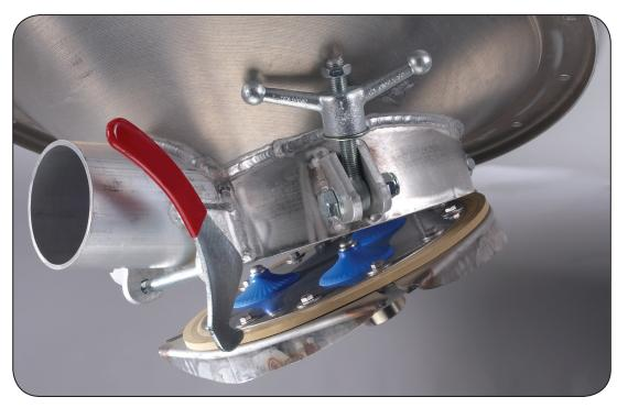
Pneumatic OR Gravity Unloading Two Way Hauling of Different Products Easy Clean Out 5" or 6" Unloading Pipes Rugged Design for Long Service Bolt On or Weld On Swing Away Bottoms offer the best in versatility for customers looking for multipurpose use of their bulk trailer. Swing Away Bottoms permit pneumatic or gravity discharge, allow for easy clean out and washing and can be used for two-way hauling of different products.
