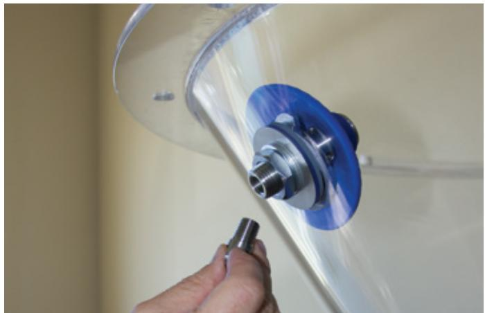
6. While continuing to hold retaining cable, slide the Fast-Fit™ sealing washer and the Fluidizer washer over the retaining cable and onto the stem. Next slide the nut over the retaining cable and thread it onto the stem.
