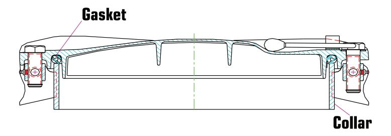
Selection Example: Assembly desired is 3/8" x 5" Aluminum collar with a viton gasket 39 + 1 (3/8" x 5" Alum) + 3 (Viton) = Assembly #3913
