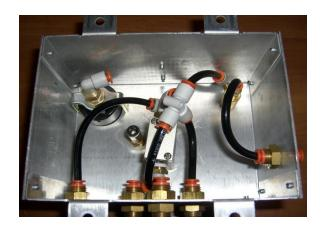
Remove the cross fitting as shown and reconnect with the tee fitting. We are no longer using the lid close indicator that will remain without a tube attached. Remove the bulkhead fitting to the green airline and save for later placement.
