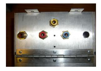
A 9/16 inch hole needs to be drilled as shown for the new yellow airline placement. You will receive a new fitting for the green line with the kit.
