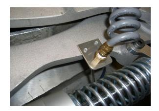
Install the provide bracket where the old pilot valve existed on the lid bottom ring. Reattach coiled airline to provided fitting. This is where the yellow airline will be attached.
