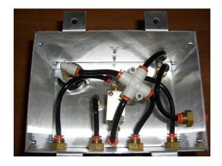
This is a view of the control box prior to the upgrade install, you will be adding additional airline; (yellow) from control box to Auto Lid.
